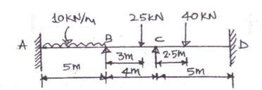
Q6) Analysis the beam as shown in fig. by stiffness matrix method. Sketch the BMD.
